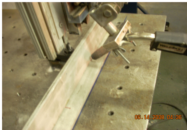
Figure 3. Close-up of Weld Setup
