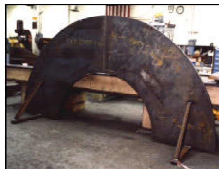
10 foot diameter disk after welding.
